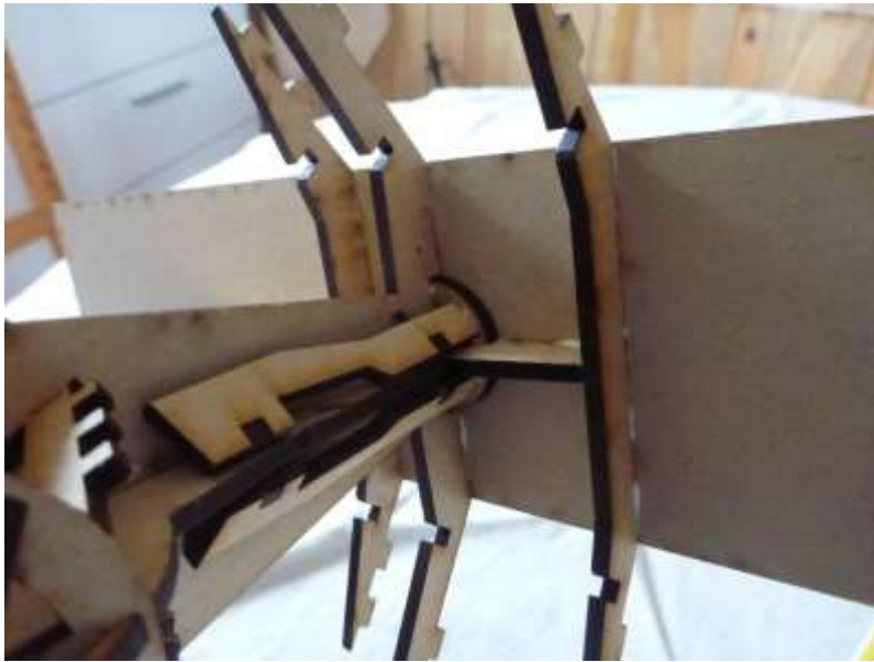
15. Attach front panel support strut.
